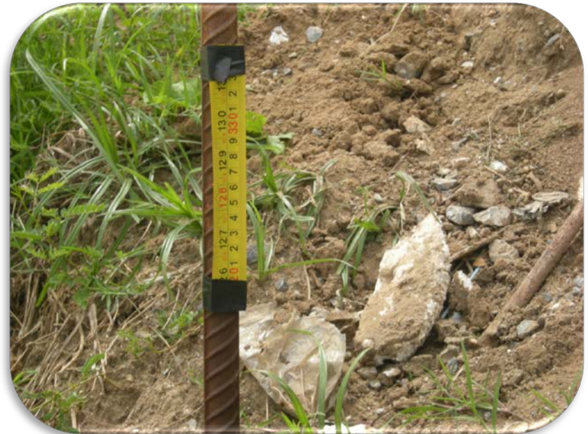
Reference BM for Leveling Measurement
