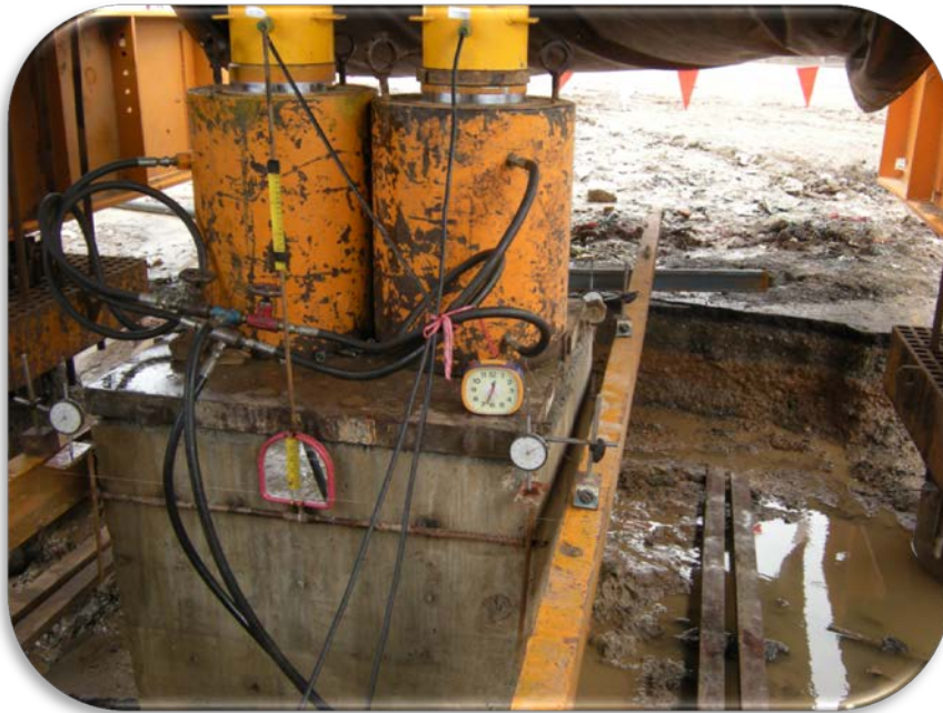
Back-up Settlement Measurement (Piano Wire & Optional Leveling)
