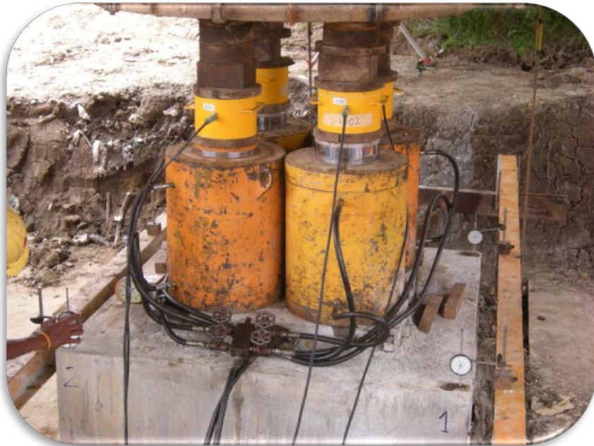
Installation Dial Gauge for Pile Settlement Measurement
