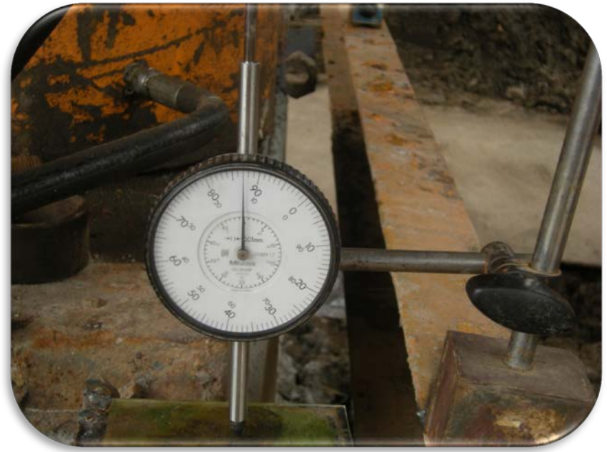
Installation Dial Gauge for Pile Settlement Measurement
